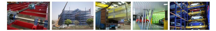
At least two of each type of machine are installed per area in the automated parking facility for redundancy. Both of the machines can perform the same tasks at the same time. Therefore, if one machine needs maintenance or repair, there is always a backup machine to keep the cars moving into and out of the garage.
