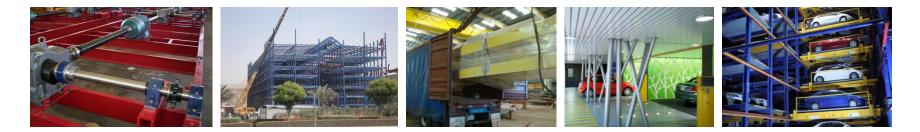
The industrial lifts, machines, pallets and the computer control systems are installed inside the supporting structure and never interfere with the façade. This gives architects a free hand in designing the external appearance of the building.
